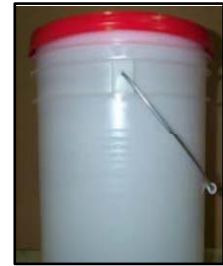
Package (parallel) improperly closed Package-(Uneven)
